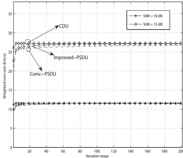
Fig. 2. Weighted sum rate vs. iteration stage for the CDU, conventional- and improved-PSDU duality algorithms for i.n.d. users when  $K = 4$ ,  $N = 32$ , and  $L = 4$  paths with an exponentially decayed PDP.
