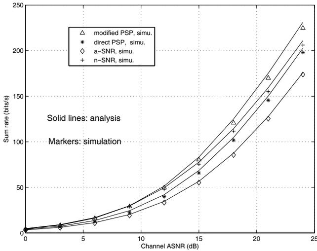
Fig. 5. Sum rate vs. channel ASNR using the PSP,  $n$ -SNR and conventional  $a$ -SNR schemes (all with EPA), assuming independent carriers and i.n.d. users,  $N = 64$  and  $K = 10$ .
