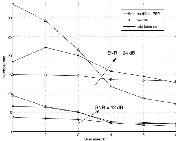
Fig. 10. Individual rate vs. user index  $k$  for several OFDMA schemes, assuming i.n.d. users with  $L = 8$  paths which have an exponentially decayed PDP,  $N = 32$  and  $K = 6$ .
