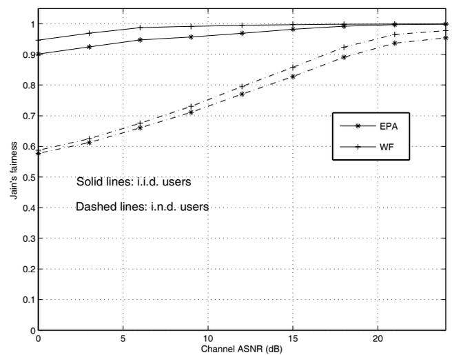
Fig. 11. Fairness index vs. channel ASNR for the rate fairness scheme with EPA and WF for i.i.d. users (furthermore with a uniform PDP) and i.n.d. users (furthermore with an exponential PDP), respectively, when  $N = 64$  and  $K = 10$ .
