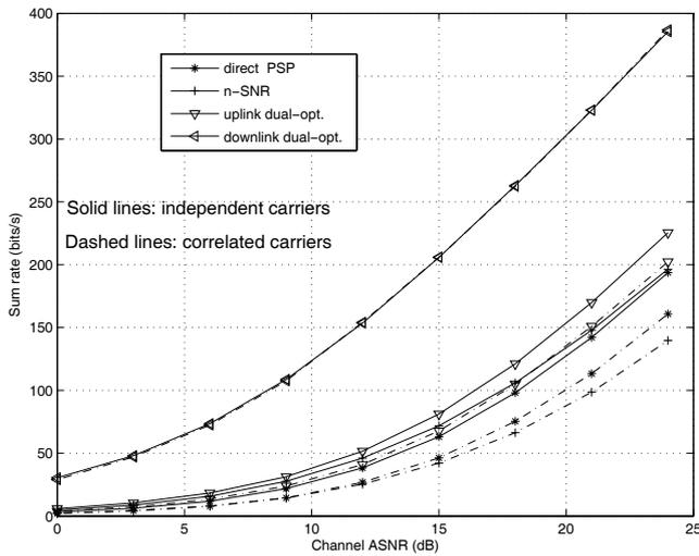
Fig. 9. Sum rate vs. channel ASNR with correlated (with an exponentially decayed PDP and  $L = 16$ ) and independent carrier channels, respectively, assuming non-i.i.d. users,  $N = 64$ , and  $K = 10$ .
