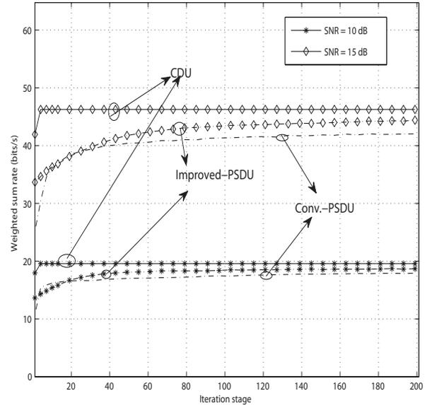
Fig. 3. Weighted sum rate vs. iteration stage for the CDU, conventional- and improved-PSDU duality algorithms for i.n.d. users when  $K = 12$ ,  $N = 32$ , and  $L = 4$  paths with an exponentially decayed PDP.
