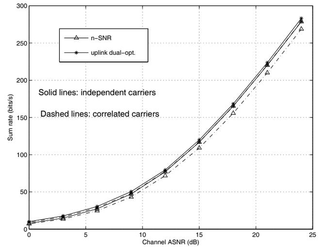
Fig. 8. Sum rate vs. channel ASNR for correlated (with a uniform PDP and  $L = 16$ ) and independent carrier channels, respectively, assuming i.i.d. users,  $N = 64$ , and  $K = 10$ .
