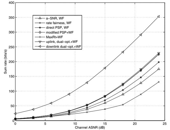
Fig. 7. Sum rate vs. channel ASNR using the proposed duality optimization, PSP,  $n$ -SNR, and rate fairness schemes (all with WF), assuming independent carriers and i.n.d. users,  $N = 64$  and  $K = 10$ .
