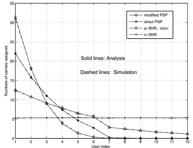
Fig. 4.  $\bar{N}_k$  vs. user index  $k$  for i.n.d. users when  $K = 12$ ,  $N = 64$ , and  $L = 16$  paths with an exponentially decayed PDP.
