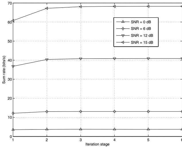
Fig. 1. Sum rate vs. iteration stage for the CDU duality algorithm for i.n.d. users, when  $K = 12$ ,  $N = 64$ , and  $L = 16$  paths with an exponentially decayed PDP.
