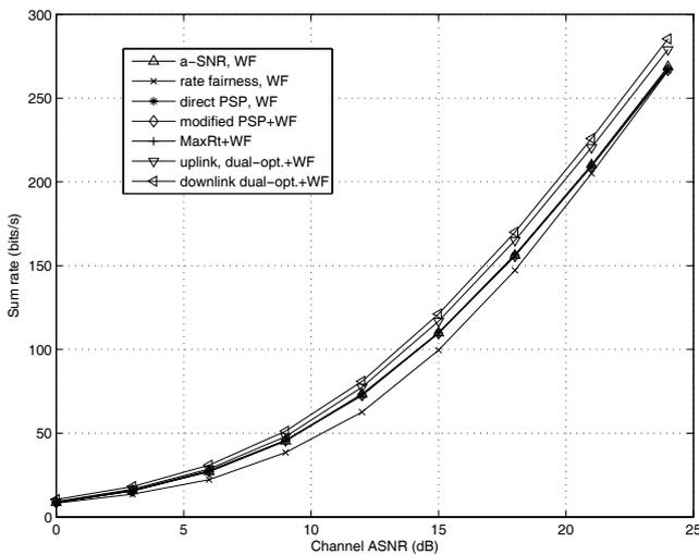
Fig. 6. Sum rate vs. channel ASNR using the proposed duality optimization, PSP,  $n$ -SNR, and rate fairness schemes (all with WF), assuming correlated carriers with exponentially decayed multipath PDP with  $L = 16$ , and i.i.d. users,  $N = 64$  and  $K = 10$ .
