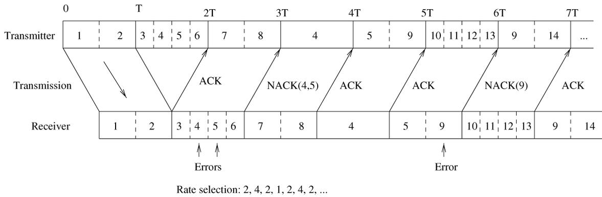
Fig. 1. SR-ARQ-based error control under variable rate transmission at the radio link level.
