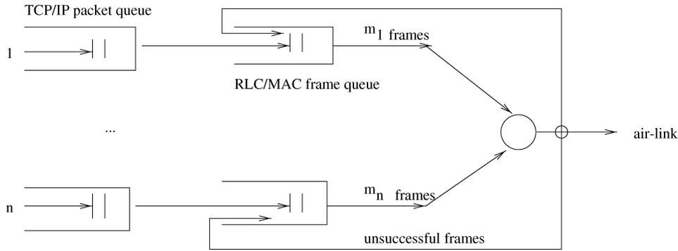
Fig. 2. Queuing of TCP/IP packets and the corresponding radio frames at the BS for downlink transmission.
