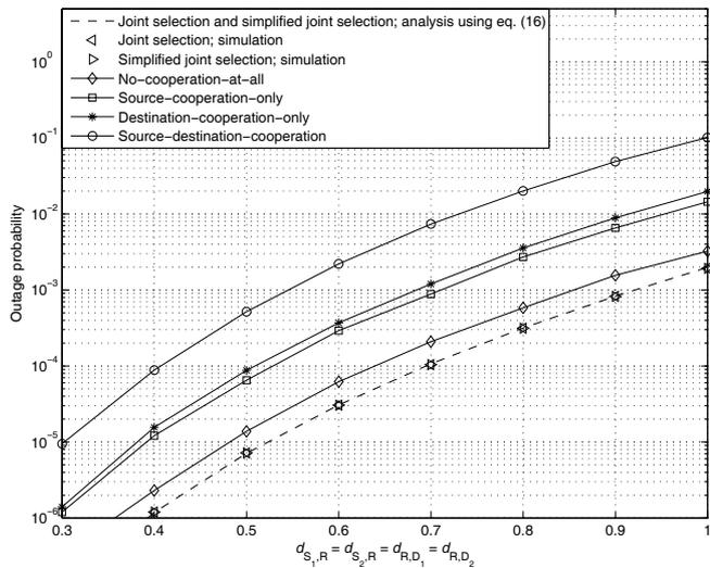
Fig. 8. Outage probabilities against  $d_{S_1,R} = d_{S_2,R} = d_{R,D_1} = d_{R,D_2}$  of the joint selection, simplified joint selection, and four end-to-end transmission strategies.  $R = 1$  bps/Hz,  $10 \log_{10} \mathcal{P} = 20$ , and  $d_{S_1,S_2} = d_{D_1,D_2} = 0.2$ .
