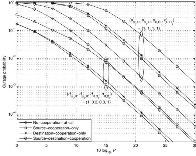
Fig. 5. Outage probabilities of the no-cooperation-at-all, source-cooperation-only, destination-cooperation-only, and source-destination-cooperation for two different channel settings:  $(d_{S_1,R}, d_{S_2,R}, d_{R,D_1}, d_{R,D_2}) = (1, 1, 1, 1)$  and  $(1, 0.3, 0.3, 1)$ .  $R = 1$  bps/Hz and  $d_{S_1,S_2} = d_{D_1,D_2} = 0.2$ .
