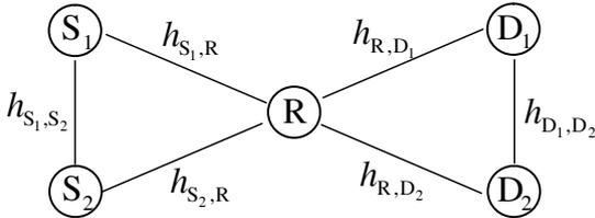
Fig. 1. System model for a cooperative diversity network consisting of two source-destination pairs and a relay without any direct-path from sources to destinations.
