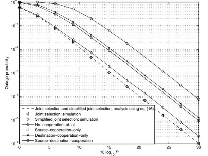
Fig. 6. Outage probabilities of the joint selection, simplified joint selection, and four end-to-end transmission strategies for a symmetric channel setting:  $(d_{S_1,R}, d_{S_2,R}, d_{R,D_1}, d_{R,D_2}) = (0.7, 0.7, 0.7, 0.7)$ .  $R = 1$  bps/Hz and  $d_{S_1,S_2} = d_{D_1,D_2} = 0.2$ .
