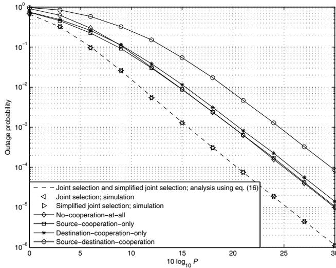
Fig. 7. Outage probabilities of the joint selection, simplified joint selection, and four end-to-end transmission strategies for an asymmetric channel setting:  $(d_{S_1,R}, d_{S_2,R}, d_{R,D_1}, d_{R,D_2}) = (1, 0.5, 0.5, 1)$ .  $R = 1$  bps/Hz and  $d_{S_1,S_2} = d_{D_1,D_2} = 0.2$ .
