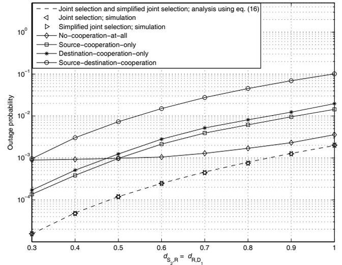
Fig. 9. Outage probabilities against  $d_{S_2,R} = d_{R,D_1}$  of the joint selection, simplified joint selection, and four end-to-end transmission strategies.  $R = 1$  bps/Hz,  $10 \log_{10} \mathcal{P} = 20$ ,  $d_{S_1,R} = d_{R,D_2} = 1$ , and  $d_{S_1,S_2} = d_{D_1,D_2} = 0.2$ .
