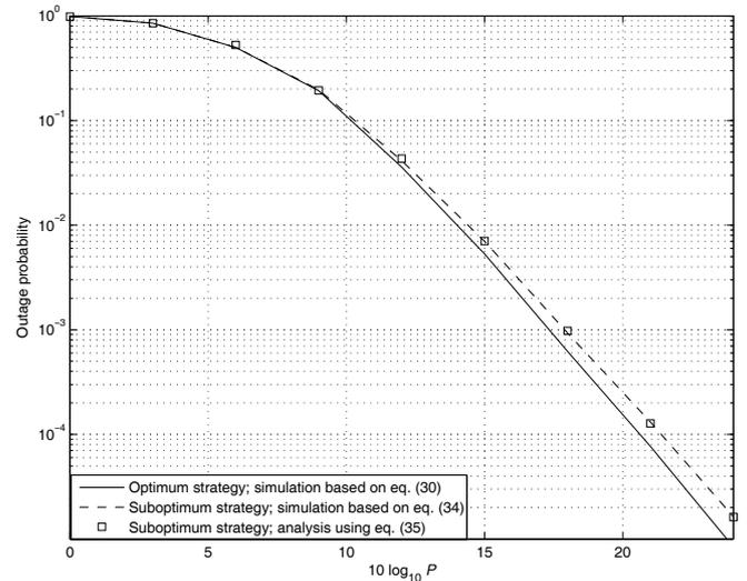
Fig. 10. Outage probabilities of the optimum strategy and suboptimum strategy for three source-destination pairs.  $(d_{S_1,R}, d_{S_2,R}, d_{S_3,R}, d_{R,D_1}, d_{R,D_2}, d_{R,D_3}) = (1, 0.7, 1.2, 0.8, 1.5, 1.2)$ ,  $(d_{S_1,S_2}, d_{S_1,S_3}, d_{S_2,S_3}, d_{D_1,D_2}, d_{D_1,D_3}, d_{D_2,D_3}) = (0.2, 0.6, 0.8, 1, 0.7, 1.2)$ , and  $R = 1$  bps/Hz.
