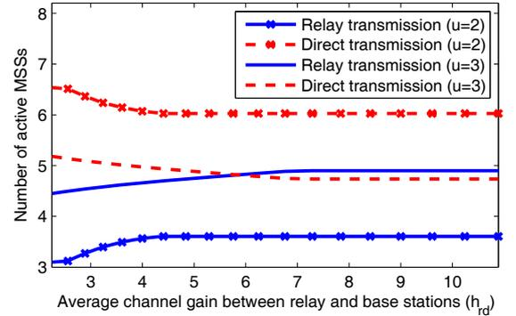
Fig. 3. The number of MSSs in a particular extended service area choosing direct and relay-based transmissions.
