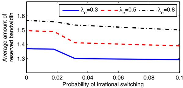
Fig. 5. Average amount of reserved bandwidth by the relay station under different probability of irrational mode switching by an MSS.
