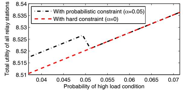
Fig. 6. Total utility of relay stations under different probability of high traffic load condition.
