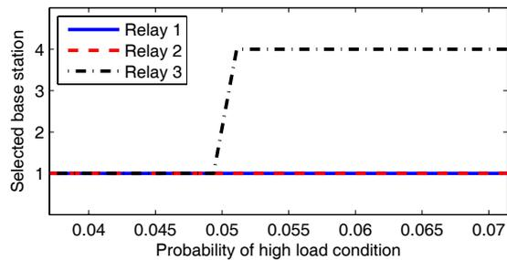
Fig. 7. Base station selection of a relay station under different probability of high arrival rate.
