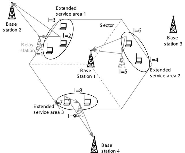
Fig. 1. System model for the MMR network.
