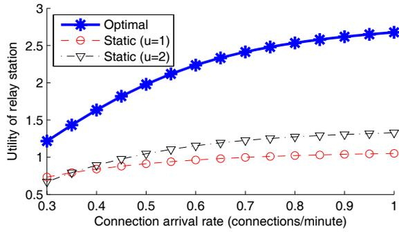
Fig. 4. Utility of a relay station under different connection arrival rate. The utility from optimal policy and static policy on bandwidth reservation and admission control are compared.
