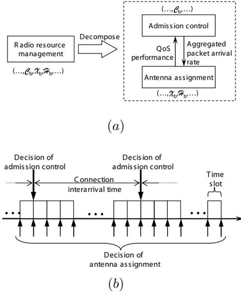
Fig. 2. (a) Decomposition of RRM problem for the wireless router and (b) decisions of antenna assignment and admission control.
