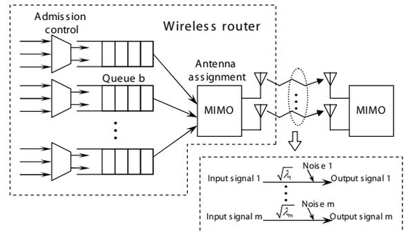
Fig. 1. System model of a MIMO-enabled wireless router with multiple traffic classes.
