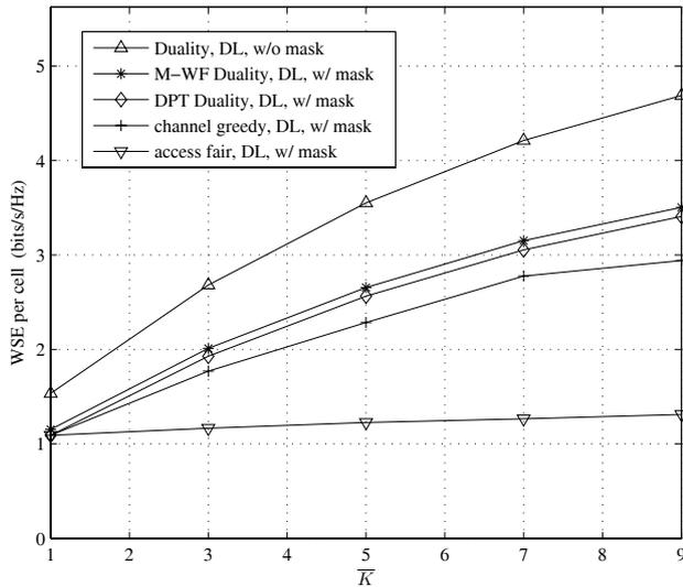
Fig. 7. WSE per cell vs.  $\bar{K}$  for several duality and multiuser diversity schemes (channel-greedy and access-fairness) in CRN downlink transmission, when  $P_T = 30$  dBm,  $N_c = 16$ ,  $P_{OP} = 0.01$  (for all  $n, m$ ), and  $P_{SOP} = 0.5$ .
