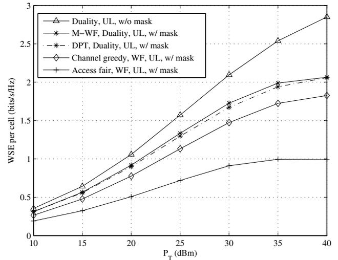
Fig. 4. WSE per cell vs. transmit power  $P_T$  for several duality and multiuser diversity schemes (channel-greedy and access-fairness) in CRN uplink transmission, when  $N_c = 16$ ,  $\bar{K} = 6$ ,  $P_{OP} = 0.01$ , and  $P_{SOP} = 0.5$ .
