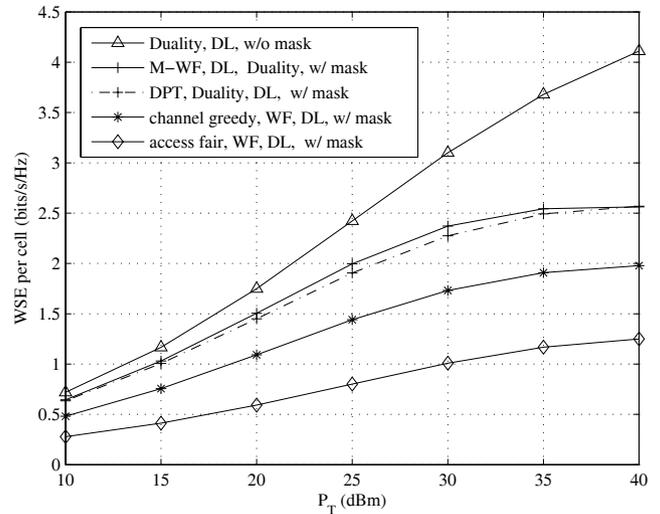
Fig. 5. WSE per cell vs. transmit power  $P_T$  for several duality and multiuser diversity schemes (channel-greedy and access-fairness) in CRN downlink transmission, when  $N_c = 16$ ,  $\bar{K} = 6$ ,  $P_{OP} = 0.01$ , and  $P_{SOP} = 0.5$ .
