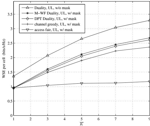
Fig. 6. WSE per cell vs.  $\bar{K}$  (number of SUs per cell) for several duality and multiuser diversity schemes (channel-greedy and access-fairness) in CRN uplink transmission, when  $P_T = 30$  dBm,  $N_c = 16$ ,  $P_{OP} = 0.01$  (for all  $n, m$ ), and  $P_{SOP} = 0.5$ .
