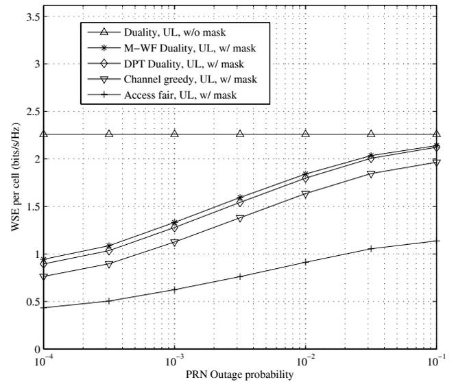
Fig. 8. WSE per cell vs.  $P_{OP}$  (target outage probability at PRN BS) for several duality and multiuser diversity schemes in CRN uplink transmission, when  $\bar{K} = 6$  per cell,  $P_T = 30$  dBm,  $N_c = 16$ , and  $P_{SOP} = 0.5$ .
