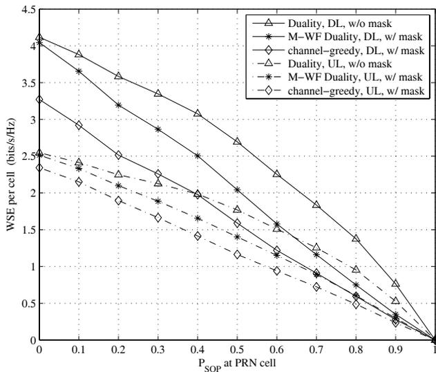
Fig. 10. WSE per cell vs. PRN subchannel occupancy probability  $P_{SOP}$  for several duality and multiuser diversity schemes in CRN uplink and downlink transmissions, when  $\bar{K} = 6$  per cell,  $P_T = 30$  dBm,  $N_c = 16$ , and  $P_{OP} = 0.01$ .
