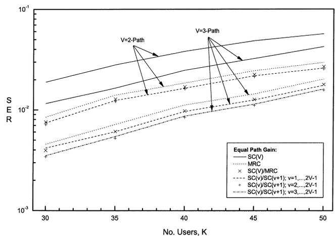
Fig. 3. SER versus  $K$  for SC( $V$ ), MRC, SC( $V$ )/MRC, and iterative SC( $v$ )/SC( $v + 1$ ) ( $v = 1, \dots, 2V - 1$ ) with uncorrelated/identical channel statistics.
