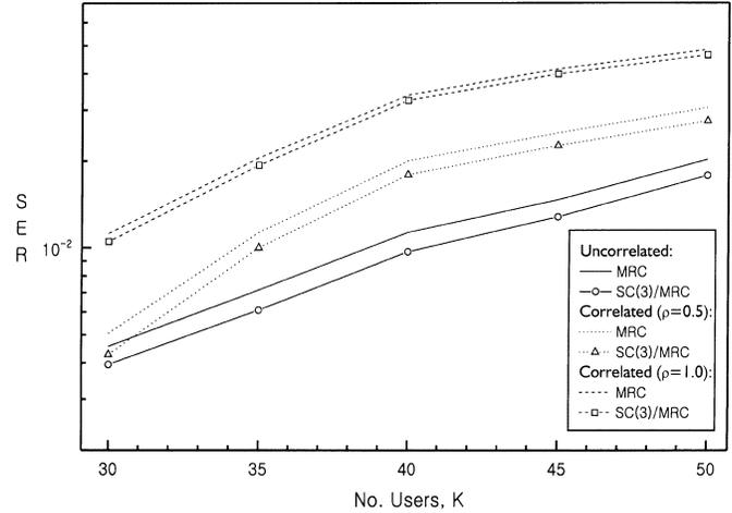
Fig. 8. SER versus  $K$  for MRC and SC(3)/MRC with correlated/identical channel statistics.
