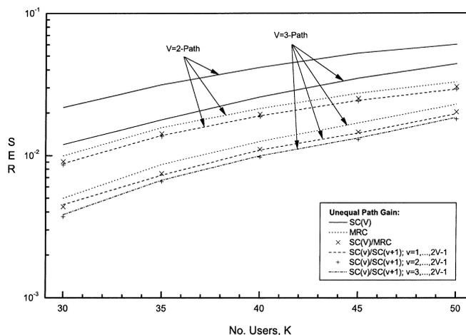
Fig. 4. SER versus  $K$  for SC( $V$ ), MRC, SC( $V$ )/MRC, and iterative SC( $v$ )/SC( $v + 1$ ) ( $v = 1, \dots, 2V - 1$ ) with uncorrelated/nonidentical channel statistics.
