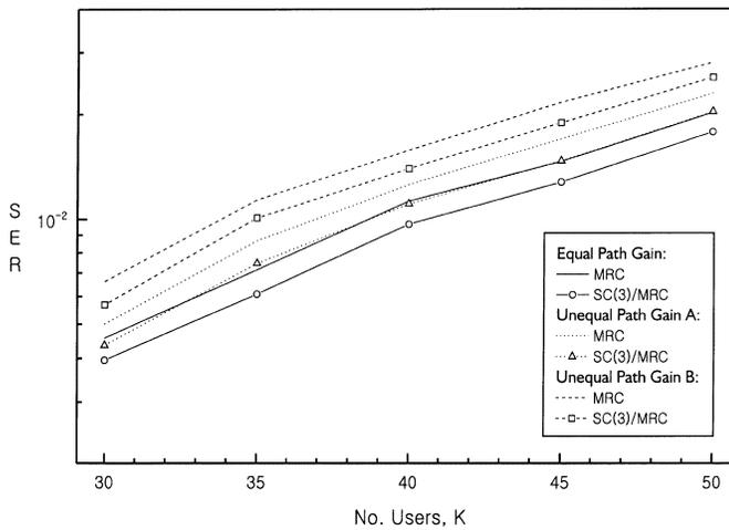
Fig. 7. SER versus  $K$  for MRC and SC(3)/MRC with uncorrelated/varying channel statistics.
