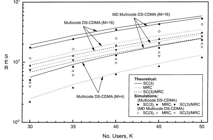
Fig. 1. SER versus  $K$  for SC(3), MRC, and SC(3)/MRC with uncorrelated/identical channel statistics.
