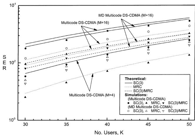
Fig. 2. SER versus  $K$  for SC(3), MRC, and SC(3)/MRC with uncorrelated/nonidentical channel statistics.
