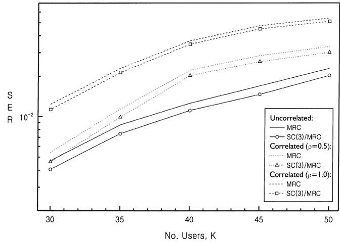
Fig. 9. SER versus  $K$  for MRC and SC(3)/MRC with correlated/nonidentical channel statistics.
