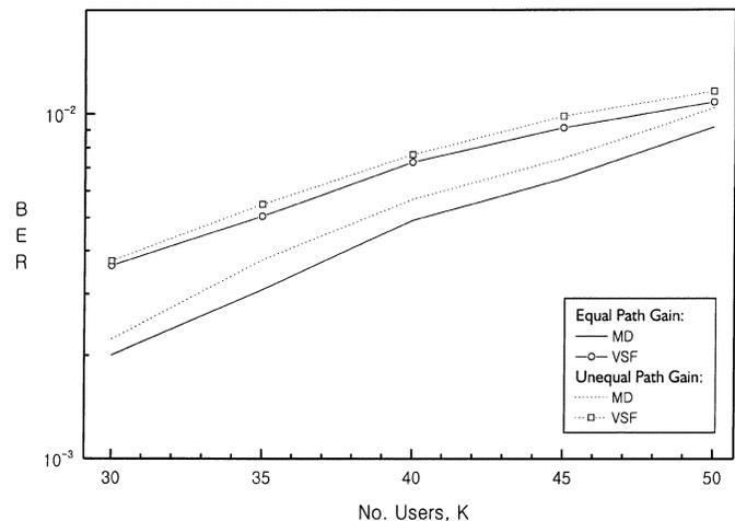
Fig. 10. BER versus  $K$  for MD (SC(3)/MRC) and VSF (MRC) with uncorrelated/identical channel statistics.
