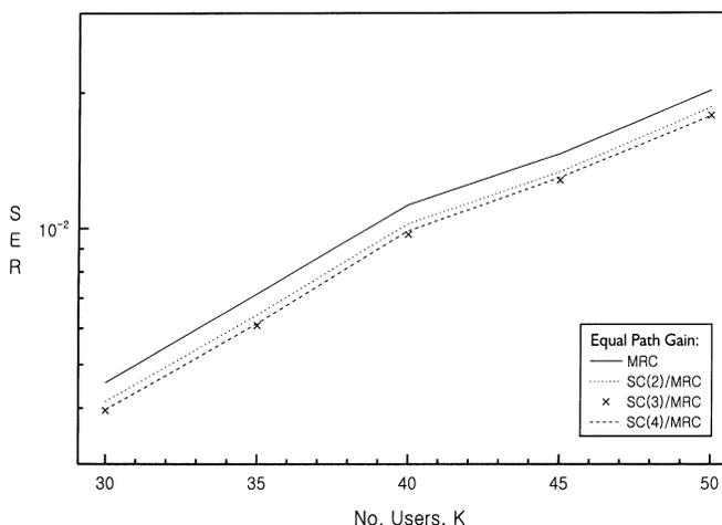
Fig. 5. SER versus  $K$  for MRC and SC( $v$ )/MRC ( $v = 2, 3, 4$ ) with uncorrelated/identical channel statistics.
