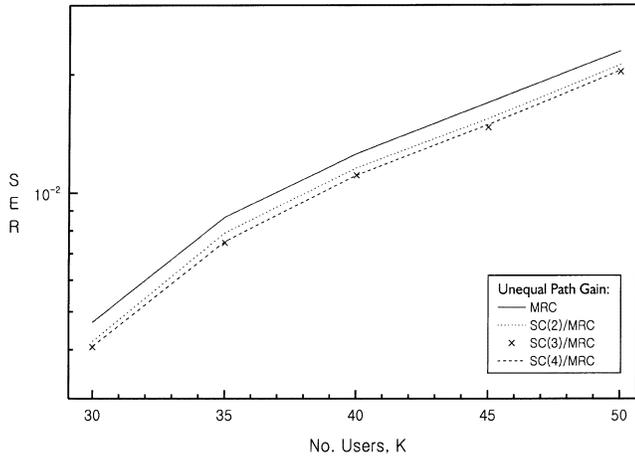
Fig. 6. SER versus  $K$  for MRC and SC( $v$ )/MRC ( $v = 2, 3, 4$ ) with uncorrelated/nonidentical channel statistics.
