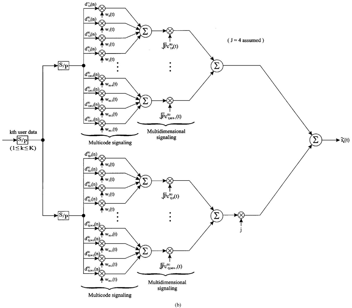
Fig. 1. (Continued.) Uplink W-CDMA system by the  $k$ th user's multidimensional signaling based on  $I$ - and  $Q$ -channel modulating sequences. (b) Multidimensional W-CDMA signaling.
