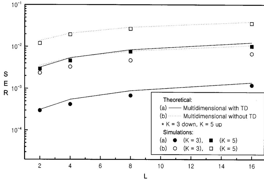
Fig. 4. SER  $P(\epsilon)$  versus  $L = 2^l$ ,  $l$  (signaling order) = 1, 2, 3, 4 when  $K = 3, 5$ ,  $M = 4$  ( $G/2 = 16$ ),  $N = 128$  and  $E/N_o = \infty$ .
