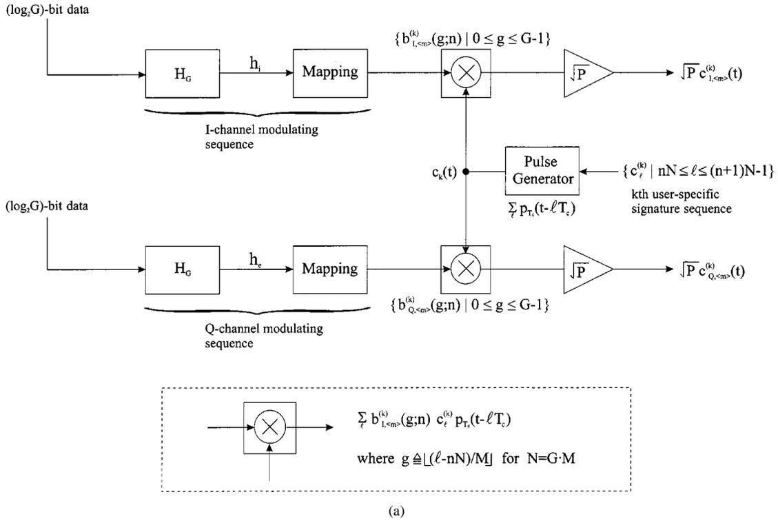
Fig. 1. Uplink W-CDMA system by the  $k$ th user's multidimensional signaling based on  $I$ - and  $Q$ -channel modulating sequences. (a) Data-modulated  $I$ - and  $Q$ -channel signature waveforms.
