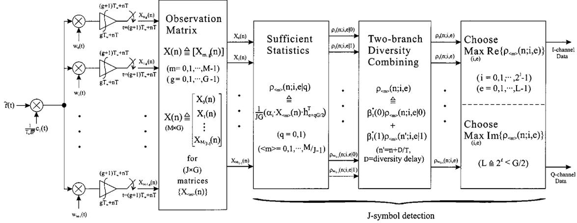
Fig. 3. Receiver structure with two-branch diversity combining and  $J$ -symbol detection for the first user.
