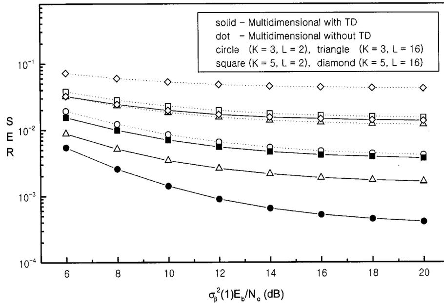
Fig. 9. SER  $P(\epsilon)$  versus  $\sigma_{\beta}^2(1) E_b/N_o$  when  $K = 3, 5, M = 4$  ( $G/2 = 16$ ),  $N = 128$  and  $L = 2, 16$ , assuming unequal average path powers with decay factor  $\epsilon = 0.3$ .
