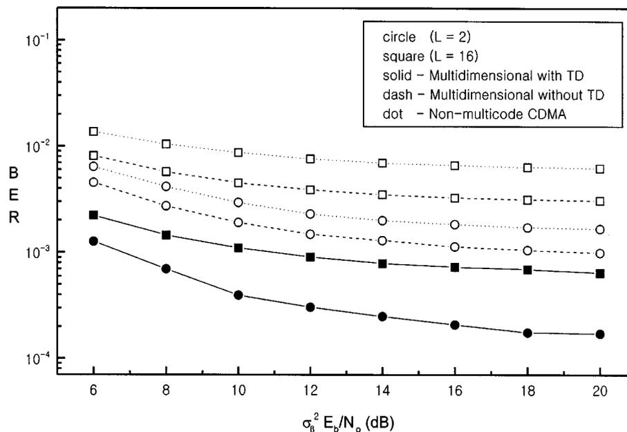
Fig. 7. BER versus  $\sigma_\beta^2 E_b/N_o$  when  $K = 3, M = 4 (G/2 = 16), N = 128$  and  $L = 2, 16$ , assuming  $N = 128 (L = 2), N = 130 (L = 4),$  and  $N = 126 (L = 8, 16)$  for the nonmulticode scheme.
