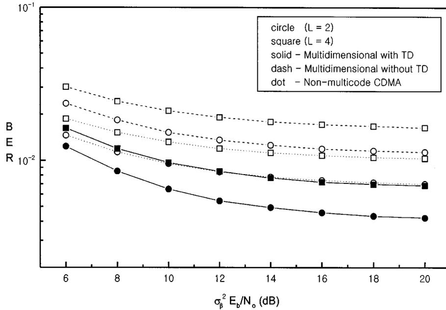
Fig. 8. BER versus  $\sigma_{\beta}^2 E_b/N_o$  when  $K = 2, M = 16$  ( $G/2 = 4$ ),  $N = 128$  and  $L = 2, 4$ , assuming  $N = 132$  ( $L = 2$ ) and  $N = 135$  ( $L = 4$ ) for the nonmulticode scheme.
