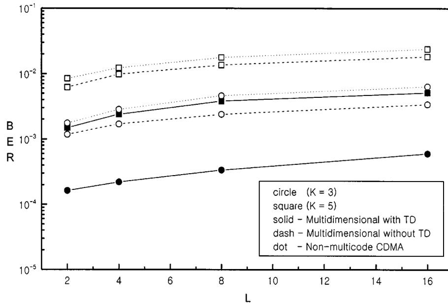
Fig. 5. BER versus  $L = 2^l$ ,  $l$  (signaling order) = 1, 2, 3, 4 when  $K = 3, 5$ ,  $M = 4$  ( $G/2 = 16$ ),  $N = 128$  and  $E/N_o = \infty$ , assuming  $N = 128$  ( $L = 2$ ),  $N = 130$  ( $L = 4$ ), and  $N = 126$  ( $L = 8, 16$ ) for the nonmulticode scheme.
