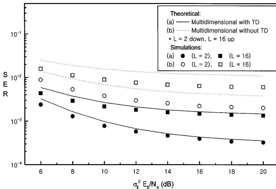
Fig. 6. SER  $P(\epsilon)$  versus  $\sigma_\beta^2 E_b/N_o$  when  $K = 3, M = 4 (G/2 = 16), N = 128$  and  $L = 2, 16$ .
