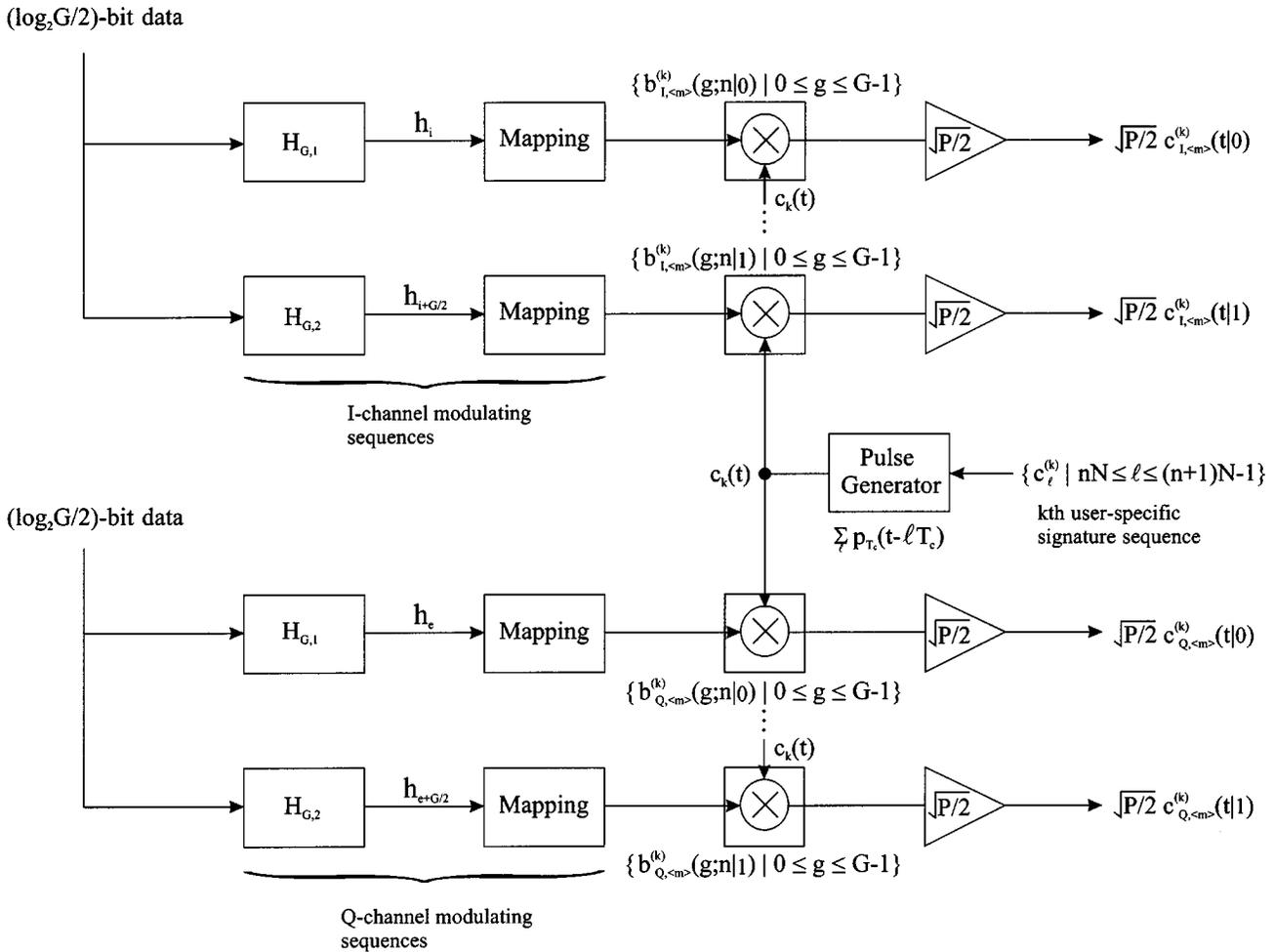
Fig. 2. Generation of data-modulated  $I$ - and  $Q$ -channel signature waveforms for two-branch transmit diversity.
