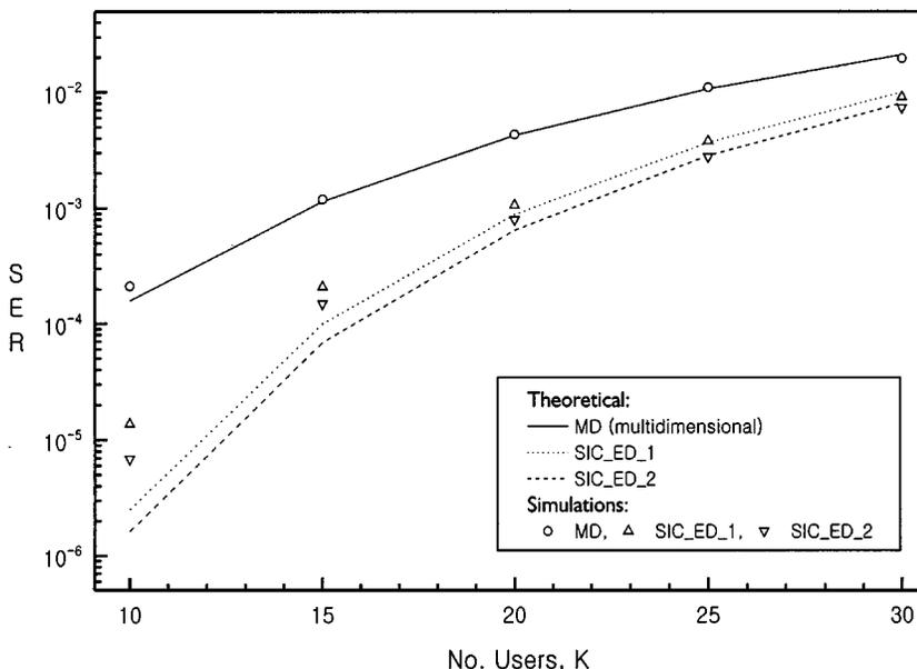
Fig. 6. SERs versus  $K$  when  $M = 16$ ,  $N = N_k = 128$ ,  $G = 8$  and  $L = 3$ , assuming three-path coherent combining.
