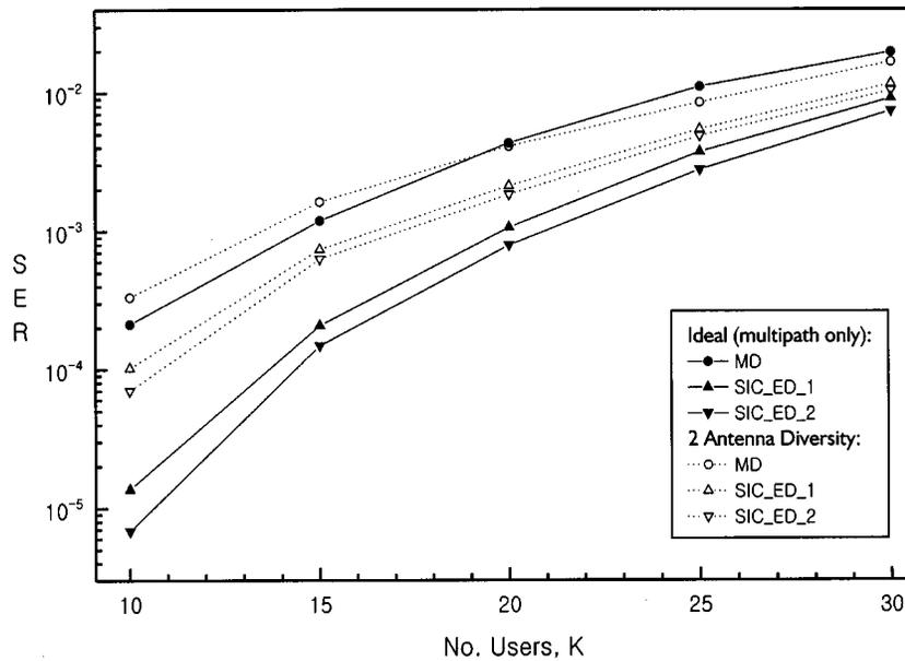
Fig. 7. SERs versus  $K$  when  $M = 16$ ,  $N = N_k = 128$ ,  $G = 8$  and  $L = 3$ , assuming three-path/2 antenna diversity combining.
