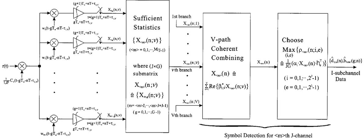
Fig. 2. Symbol-by-symbol detection of  $J$ -channel MD multicode signals.
