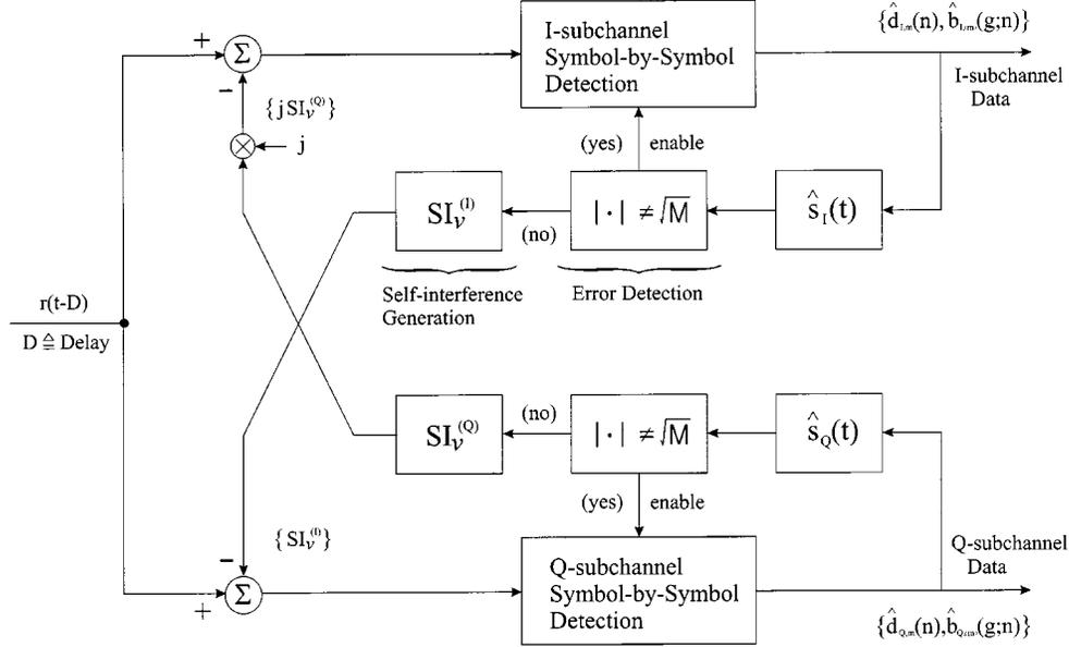
Fig. 4. Receiver structure with  $I/Q$  SI cancellation and error detection.
