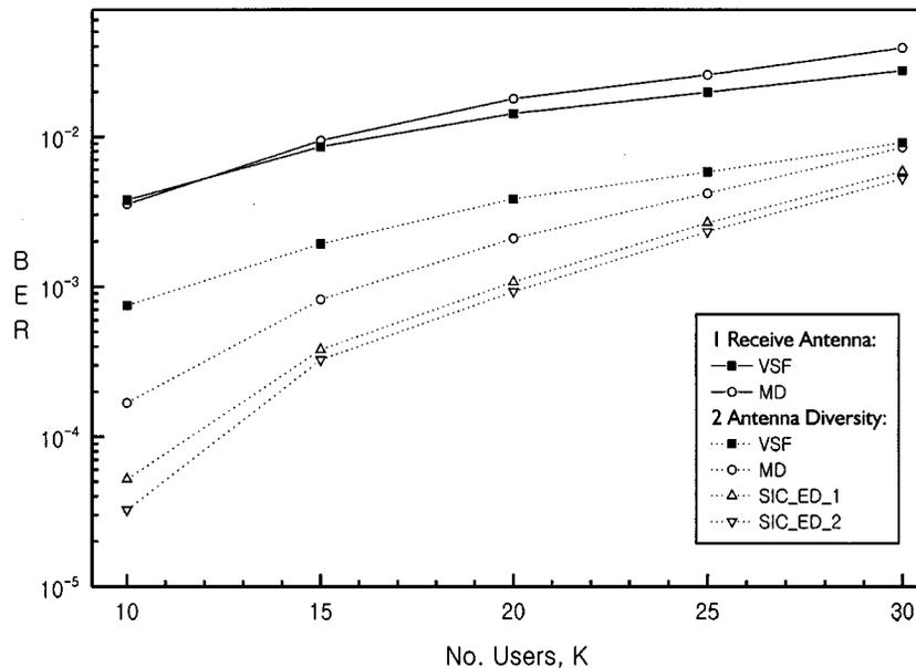
Fig. 8. BERs versus  $K$  when  $M = 16$ ,  $N = N_k = 128$ ,  $G = 8$  and  $L = 3$ , assuming three-path/2 antenna diversity combining.
