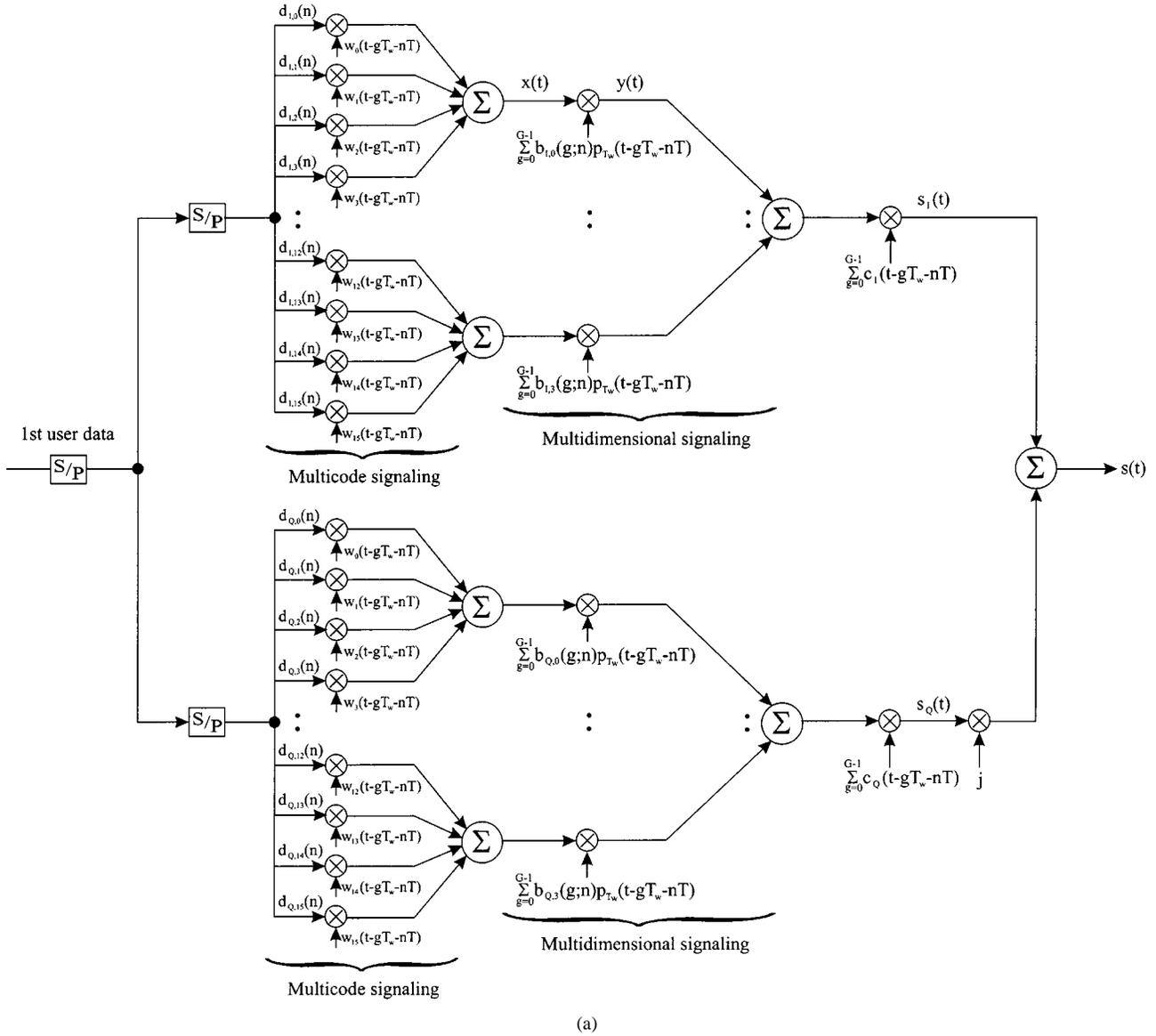
Fig. 1. MD multicode DS-CDMA signaling for a high rate user. (a) Block diagram ( $M = 16, J = 4$ ).
