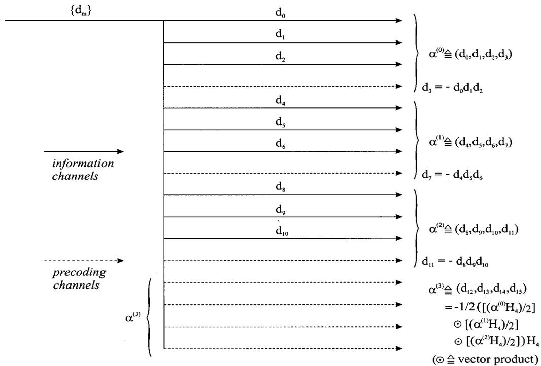
Fig. 3. Precoding for a constant envelope multicode signal when  $M = 16$  and  $J = 4$ .
