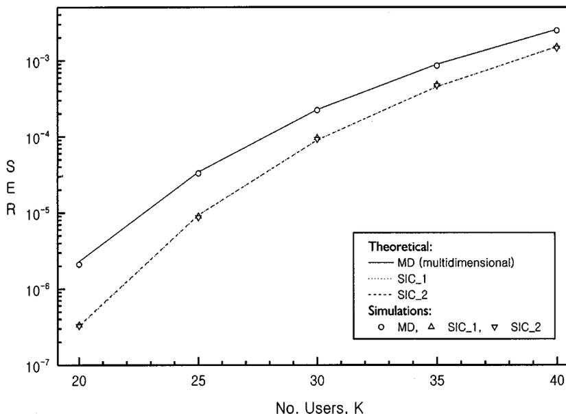
Fig. 5. SERs versus  $K$  when  $M = 4$ ,  $N = N_k = 128$ ,  $G = 32$  and  $L = 5$ , assuming three-path coherent combining.
