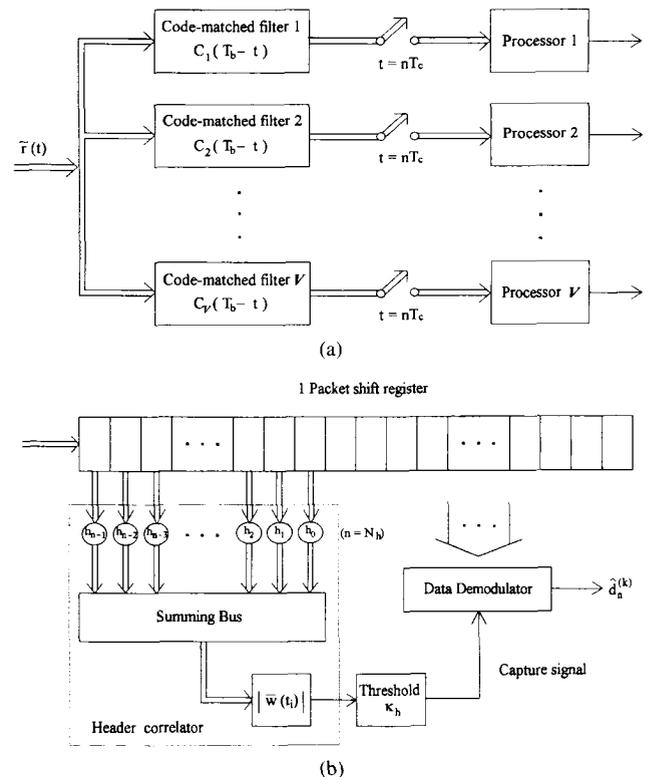
Fig. 1. Central receiver employing  $V$  different spreading codes. (a) Central receiver block diagram. (b) Realization of the processor.
