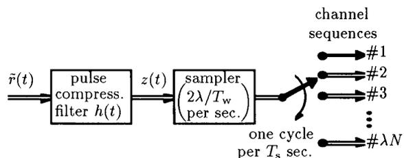
Fig. 1. Block diagram of receiver processing, illustrating the formation of channel sequences.
